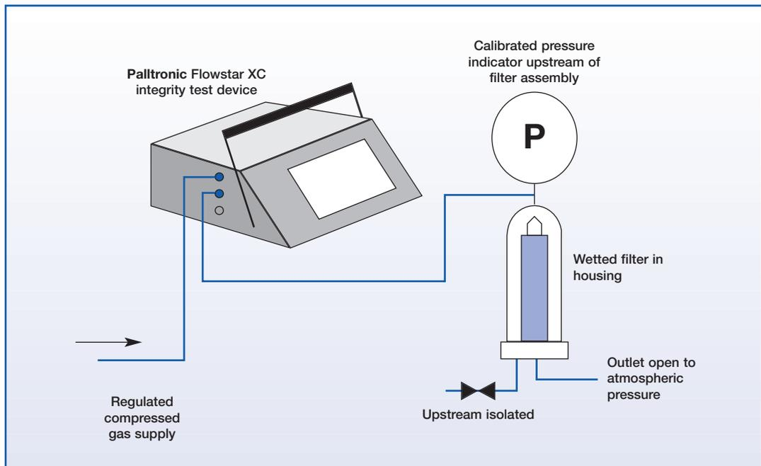
The aim of this study was to demonstrate the microbial removal efficiency of typical **Fluorodyne** EX filter cartridges in liquid challenge tests using *Brevundimonas diminuta* (ATCC 19146) and to document the correlation of the integrity test parameters to the microbial removal efficiency.
