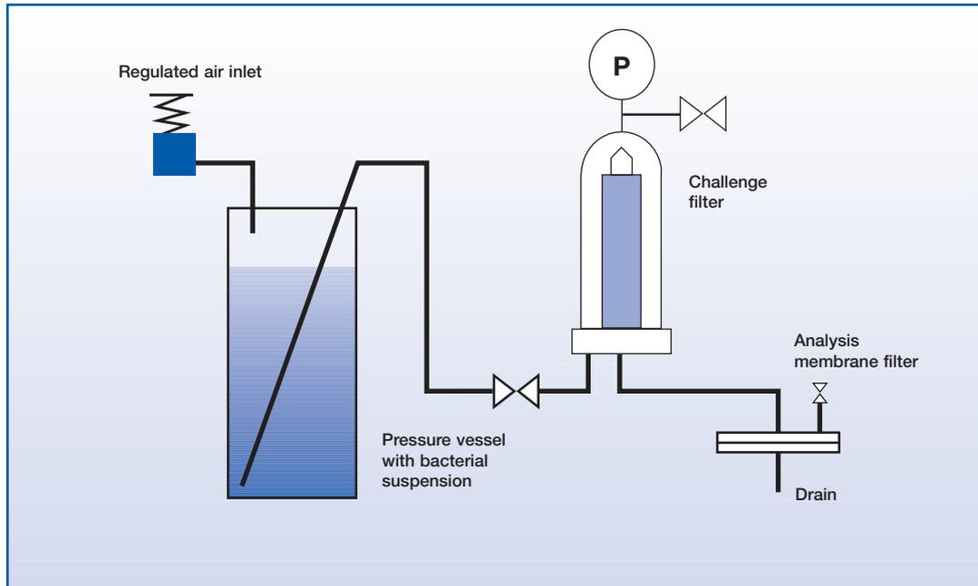
An aqueous suspension of *B. diminuta* was passed through the filter to achieve a total challenge level of  $\geq 1 \times 10^7$  colony forming units (CFU).
