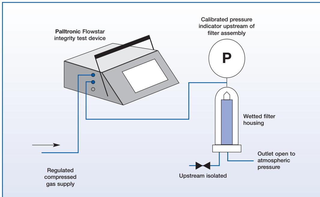
During this study **Supor** UEAV filters were wetted with deionized (DI) water at a flow rate of 10 L/min for 10 minutes and the Forward Flow values were determined using a **Palltronic** Flowstar integrity test instrument. A test pressure of 2060 mbar (30 psi) was used and the test gas was compressed air.
