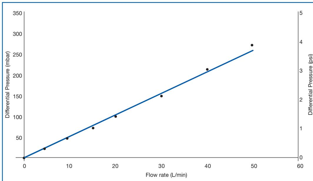
**Table 4-1 Water Flow/Differential Pressure Characteristics of Supor UEAV Filters, Part Number AB1UEAV7PH4**
