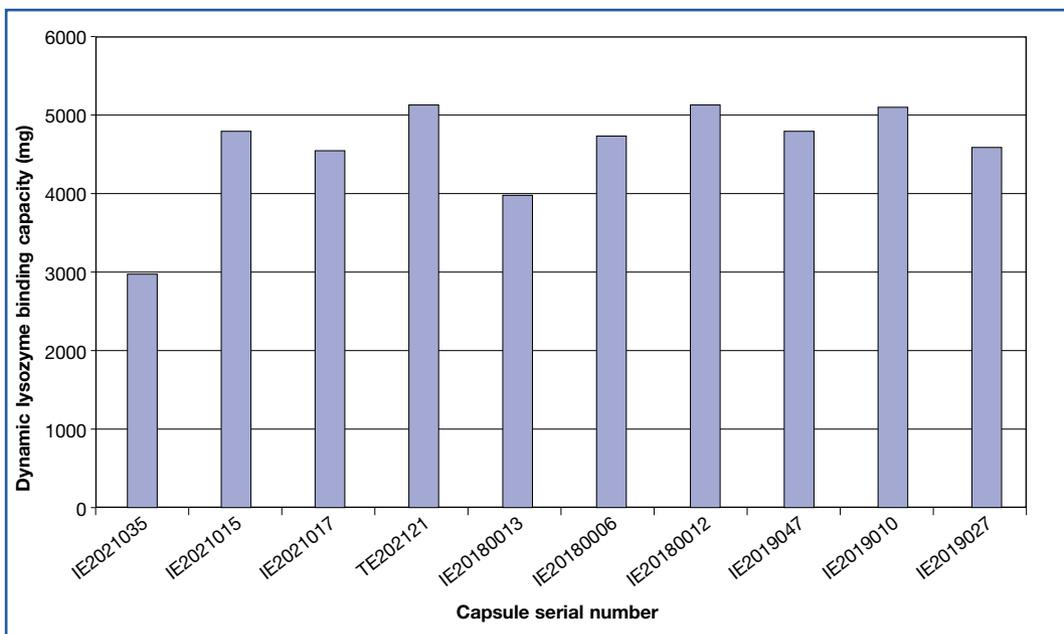
**Figure 2-3. Dynamic lysozyme binding capacity for Mustang S capsules, part number NP6MSTGSP1**
