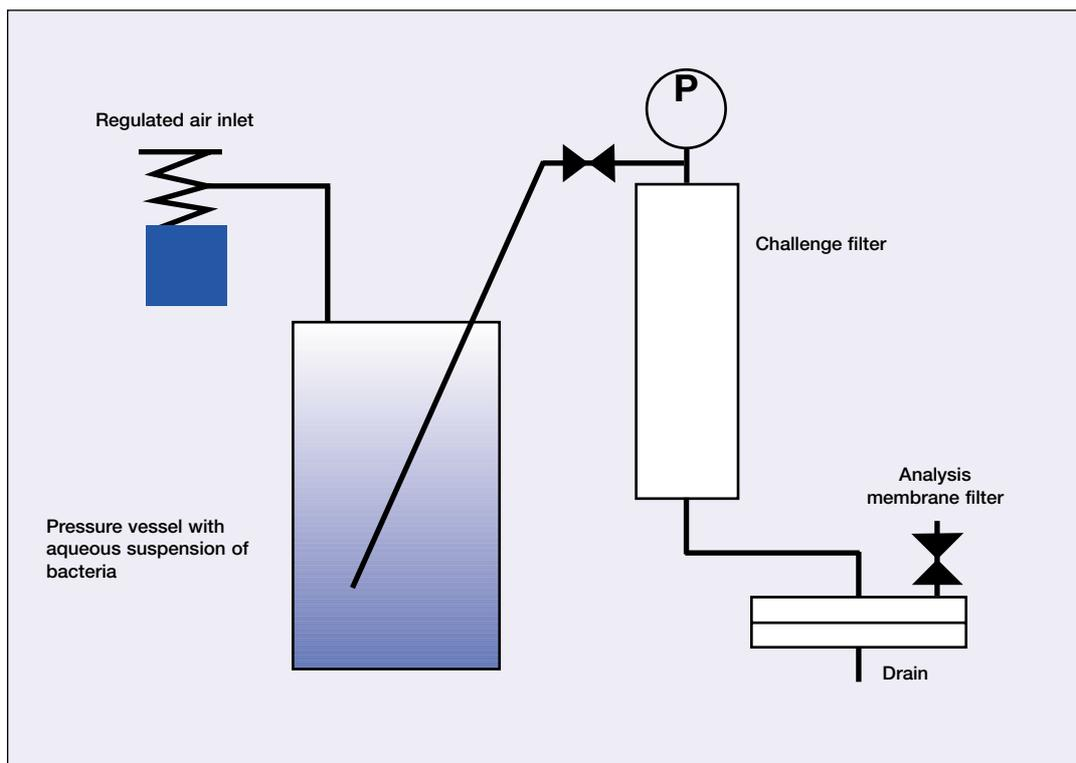
Figure 6-1. Bacterial challenge apparatus
