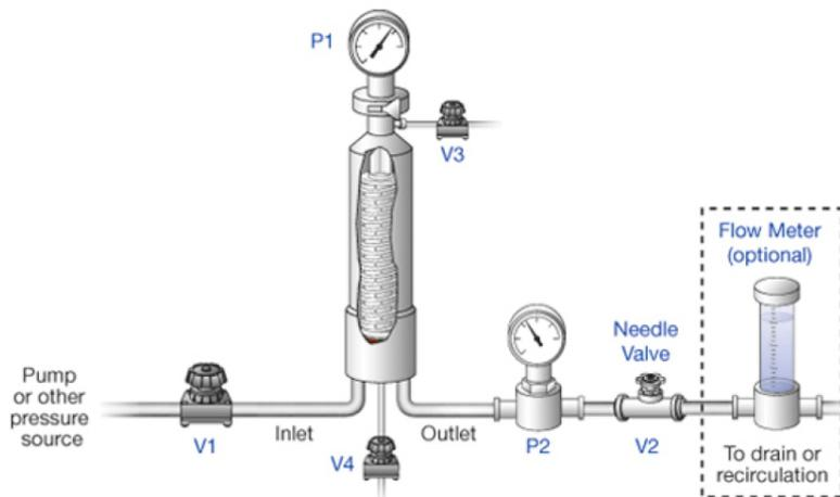
1. Start with all valves closed. Open inlet V1, and vent V3 valves.
